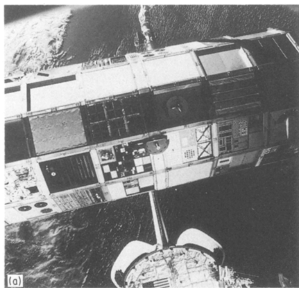
Figure 2 NASA documentary photographs of the LDEF recovery. (a) LDEF was held in the grasp of Columbia 's remote manipulator system and rotated repeatedly to accommodate an extensive photo survey. The Atlantic Ocean is in the background. (b) Suspended above the payload bay of the Space Shuttle Columbia , the LDEF is monitored by technicians during its move from the Space Shuttle to a transportation canister.
